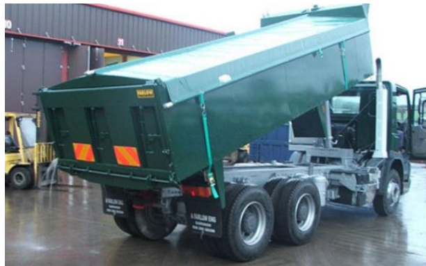
Figure 3 – Example of sheeting on lorries for removal of excavation material.
