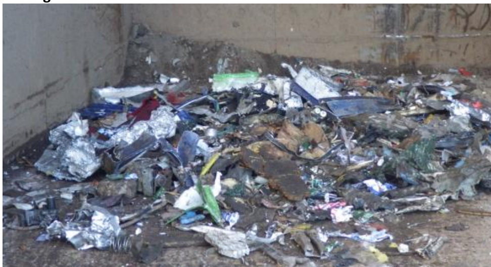
Figure 8 Undersize/non-ferrous/sterile from large vibrating screen and rotating drum magnet
