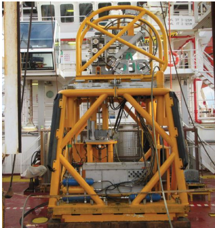
Figure 4.3: Typical Set Up for SCPT in Downhole Mode (source: Fugro)
