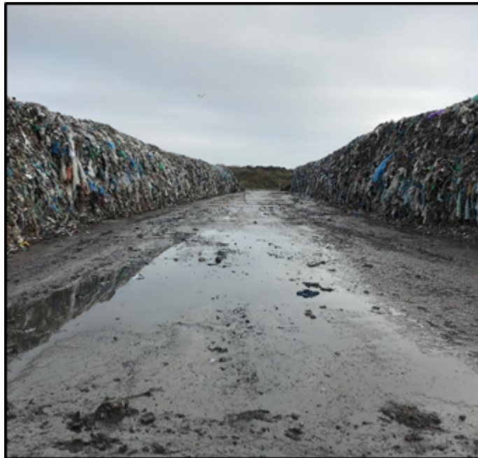
Picture 4 – showing the separation distance between RDF stacks in Field 1
