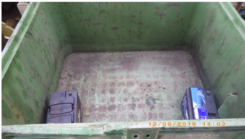
Batteries stored without a lid and damage to sidewall (bottom right of photograph)
