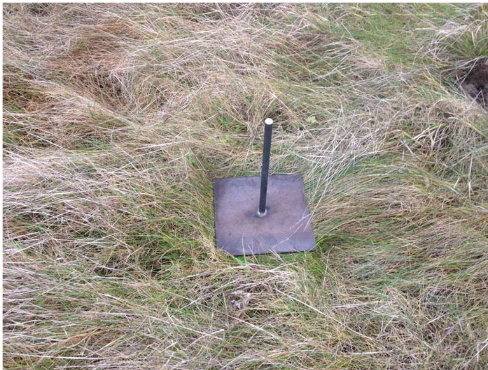
Permanent Settlement Marker on MCL (Before Installation)
