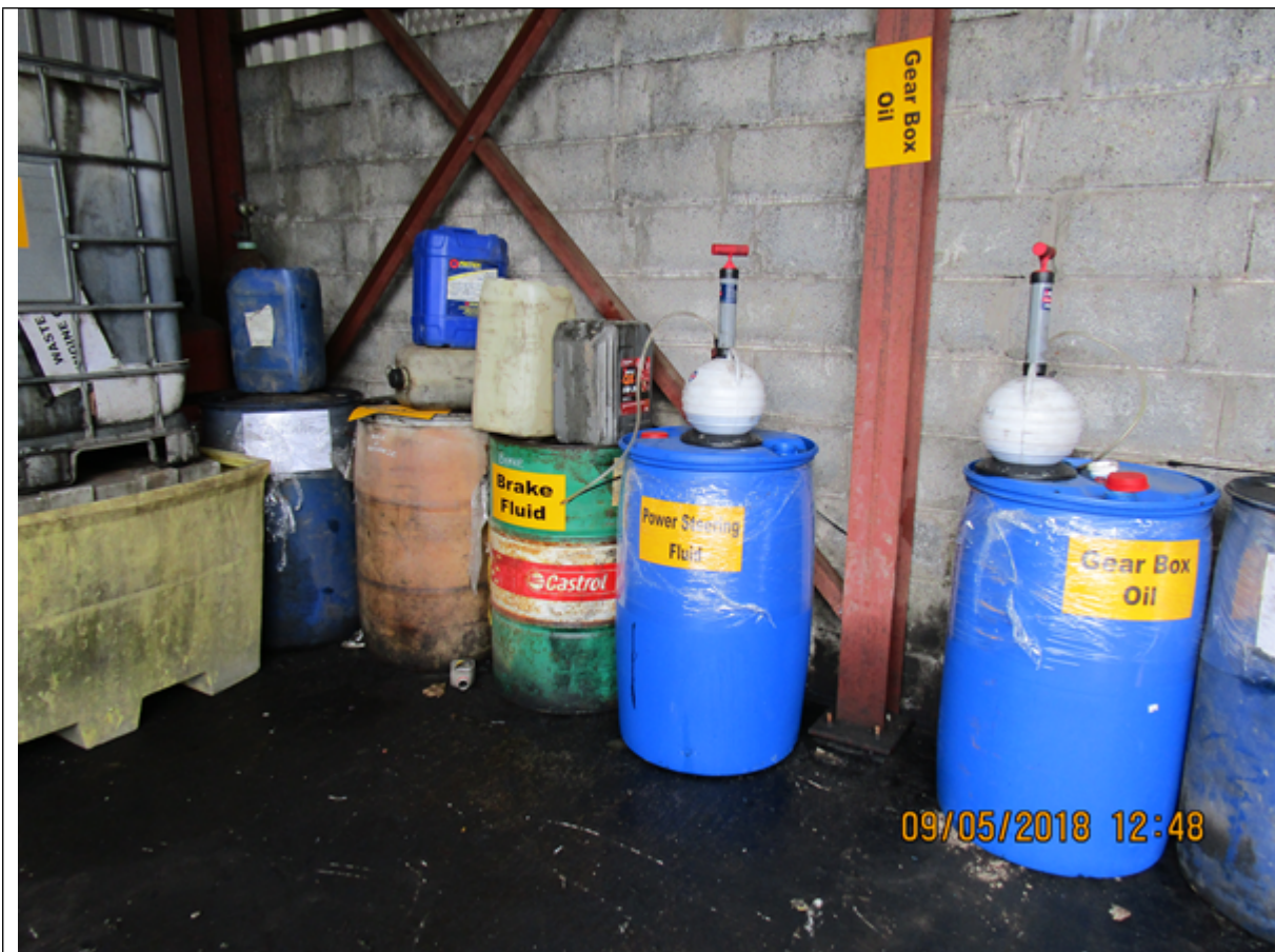
Photo showing the signage on containers and the bunding beneath the IBC
