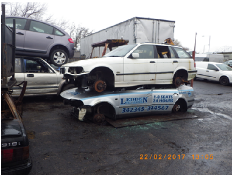
Depolluted cars stored on the interceptor
