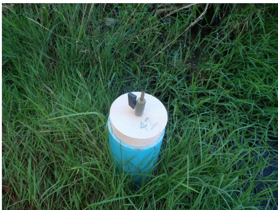
Photograph showing monitoring point 41, with gas tap left open.
