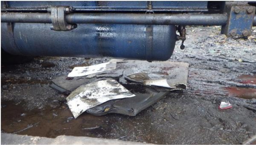
Photo showing oil absorbent pads on ground underneath mobile baler
