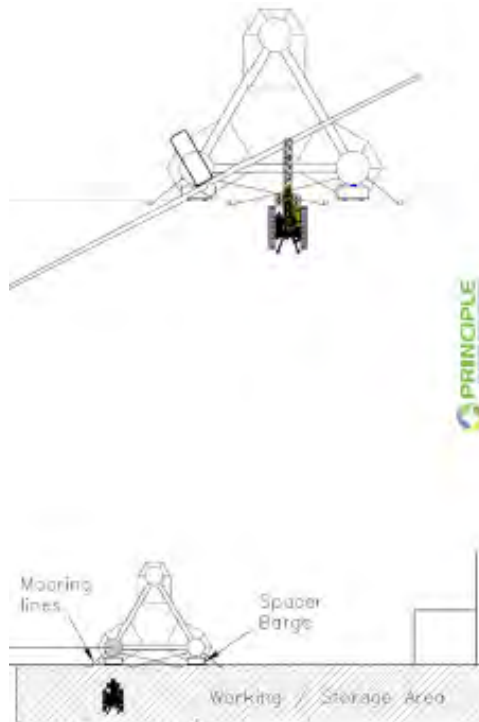
Figure 4.11: Towing out of WindFloat Unit to Offshore Array Site (source: PPI, 2019b)
