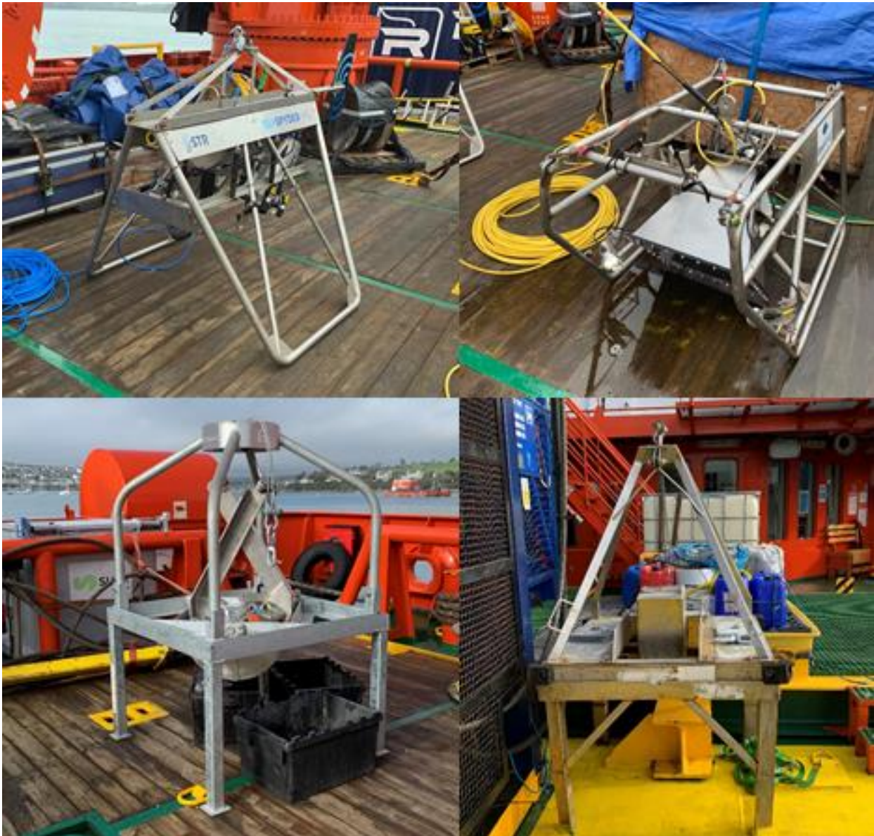
Figure 15: Top left: STR SeaSpyder camera system. Top right: OEL's ROVTECH camera system equipped with CLOC. Bottom left: Dual Van Veen grab sampler. Bottom right: Mini-Hamon grab sampler.
