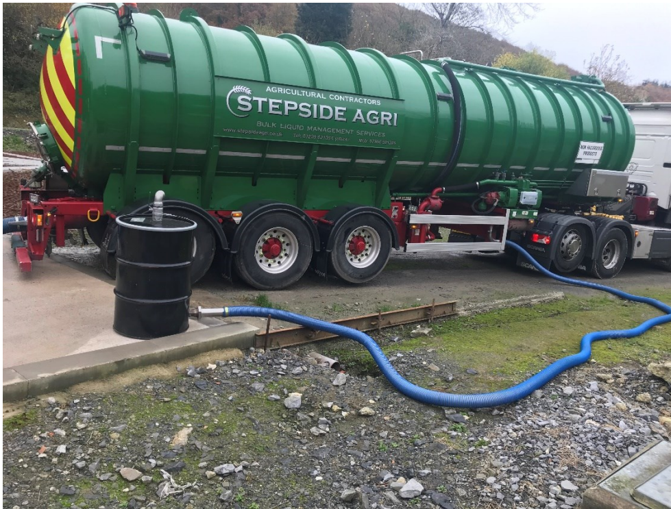
Figure A2.1: Carbon Odour Control Unit Operating during Tanker Export
