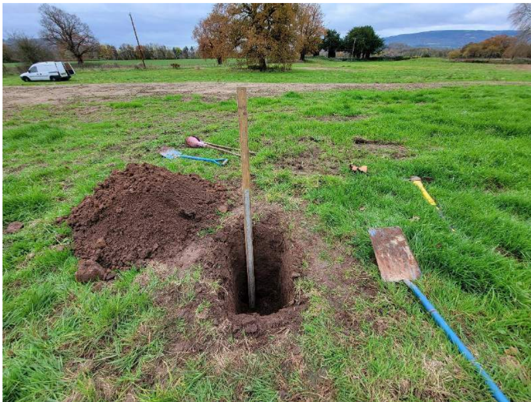
Picture 3 – Test Pit 2 Soil strata
