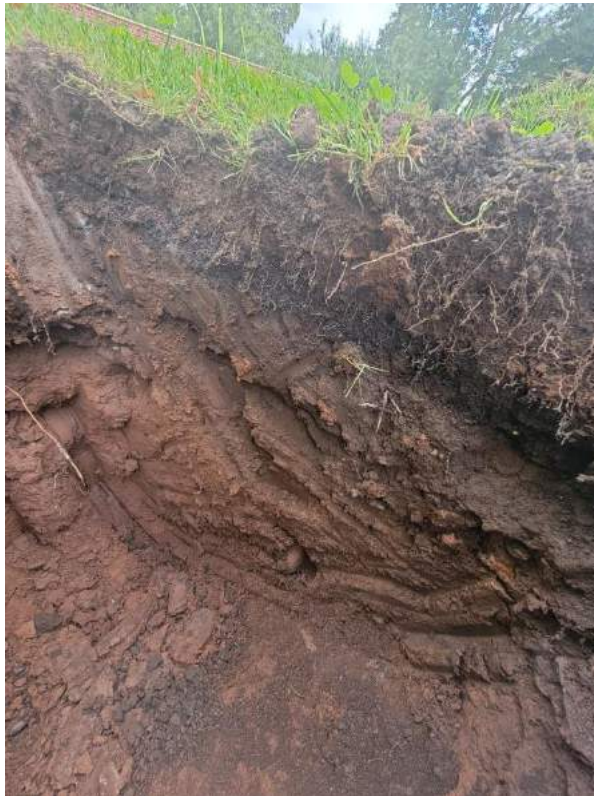
Picture 3 – Test Pit 2 Ground Strata's
