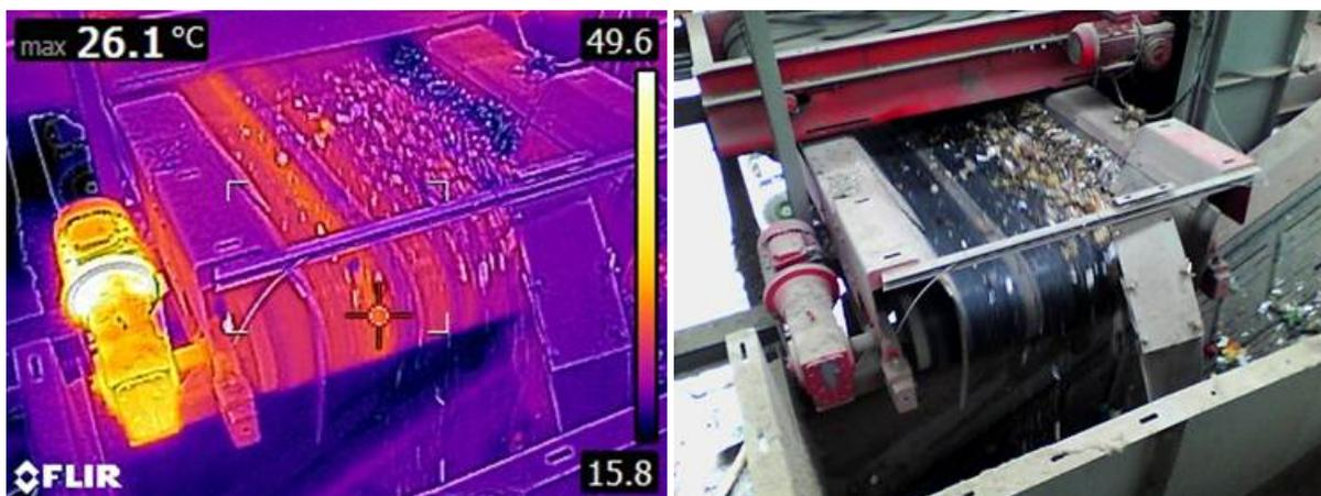
The photographs above show the temperature that the motors reach while operating. Following the end of each day each the treatment process is run for 30 minutes without any waste being fed in to it. This ensure there is no waste within the treatment process that could come in to contact with any hot parts such as motors. DPCL also undertake deep cleans of the equipment on a weekly basis to ensure there isn't a build up of material within the process.
