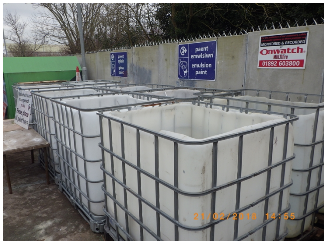
Paint storage (open-topped IBC's with no cover, and rainwater collecting in the containers)
