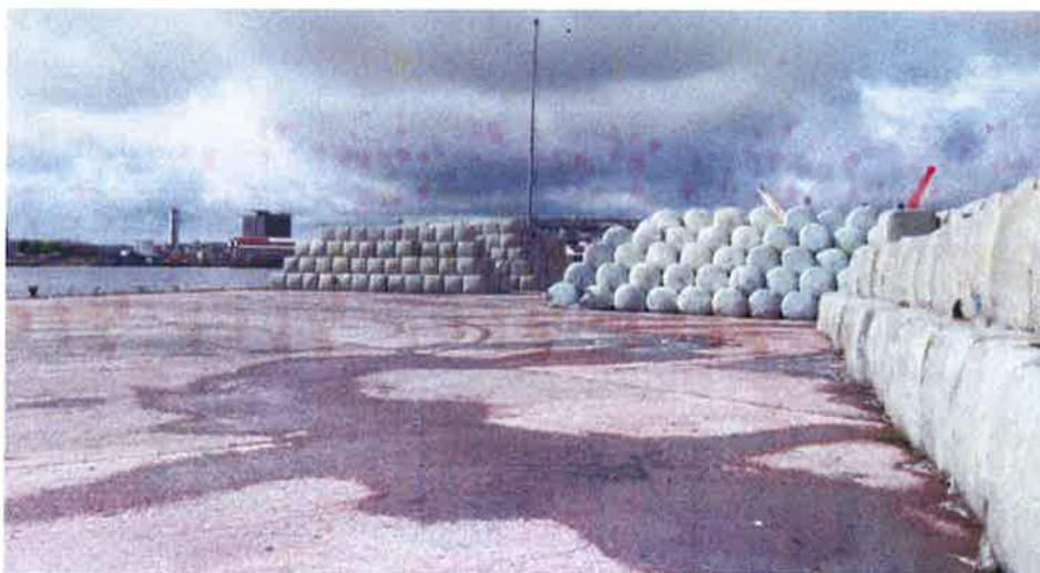
Photograph 3.1: Baled RDF and SRF Waste
