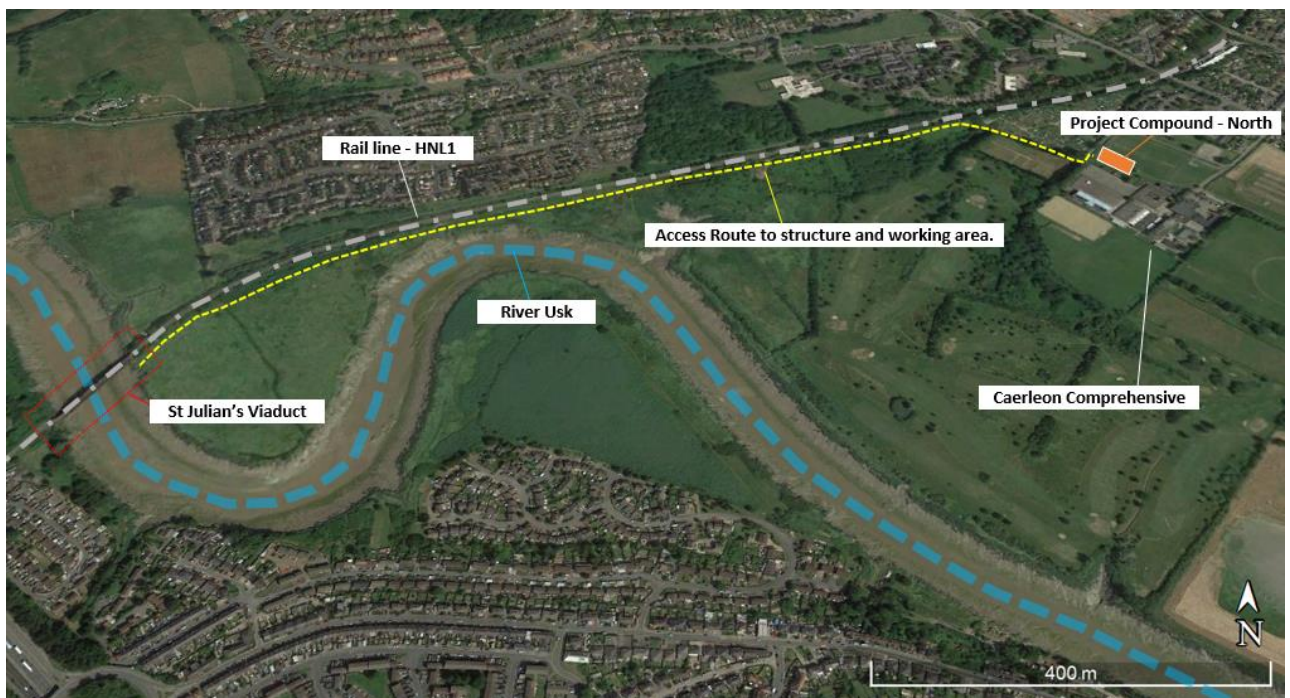
Figure 4: Northern Compound and Access Route.
