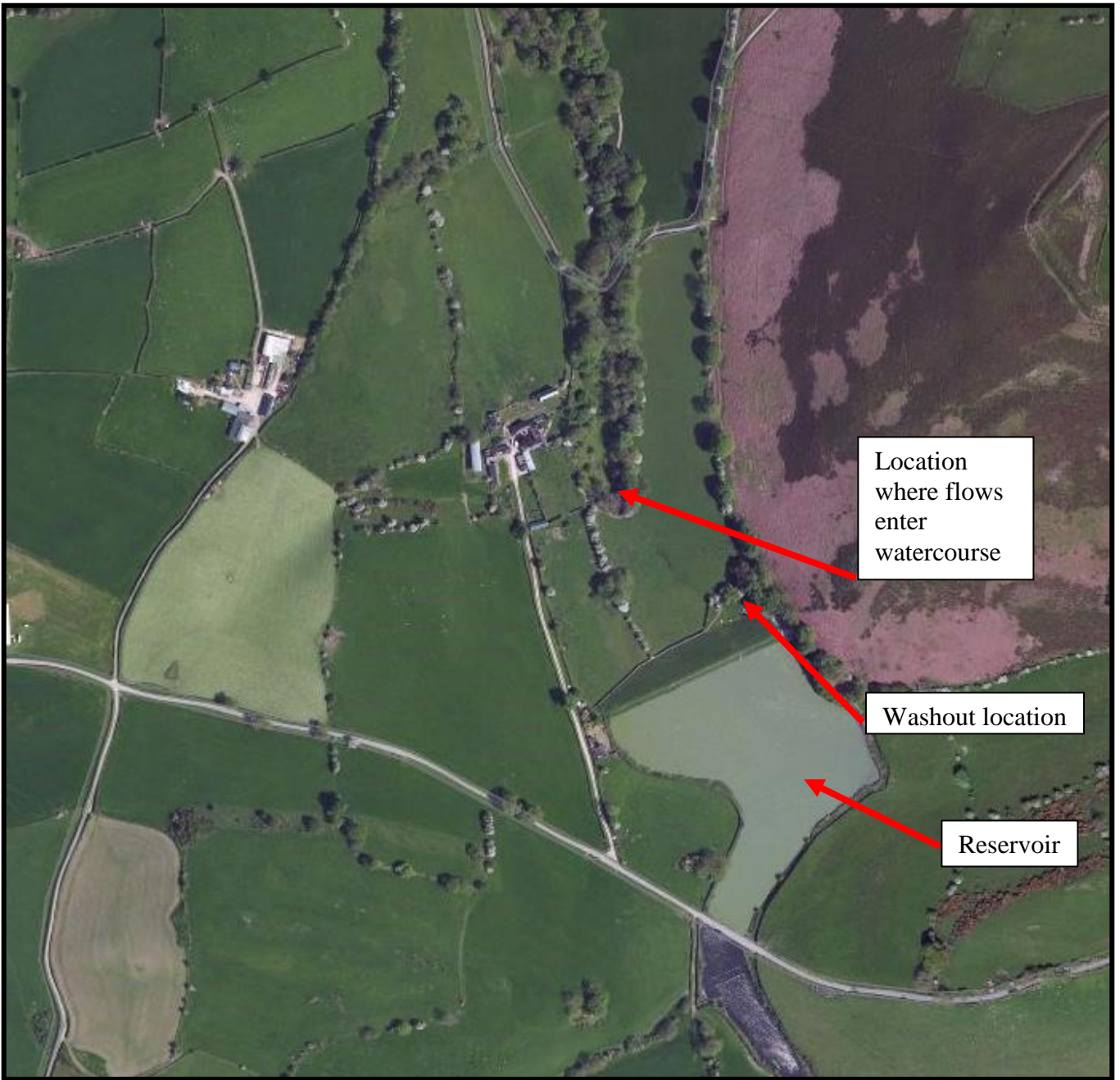
Figure 2 - location map of site with washout position and location where culvert enters stream.
