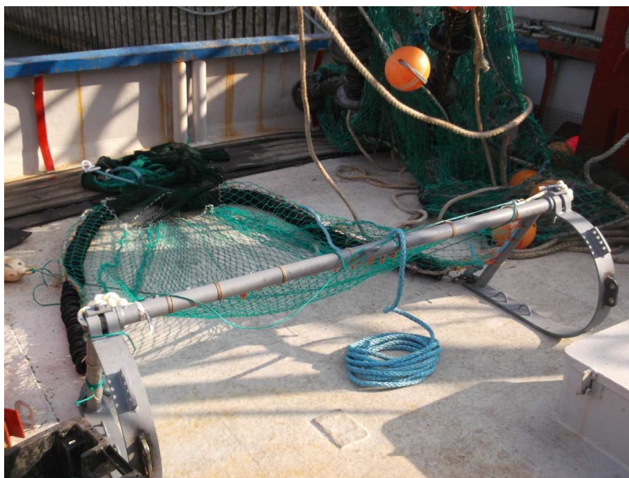
Plate 3. Standard design beam trawl used in the surveys (1.5m)
