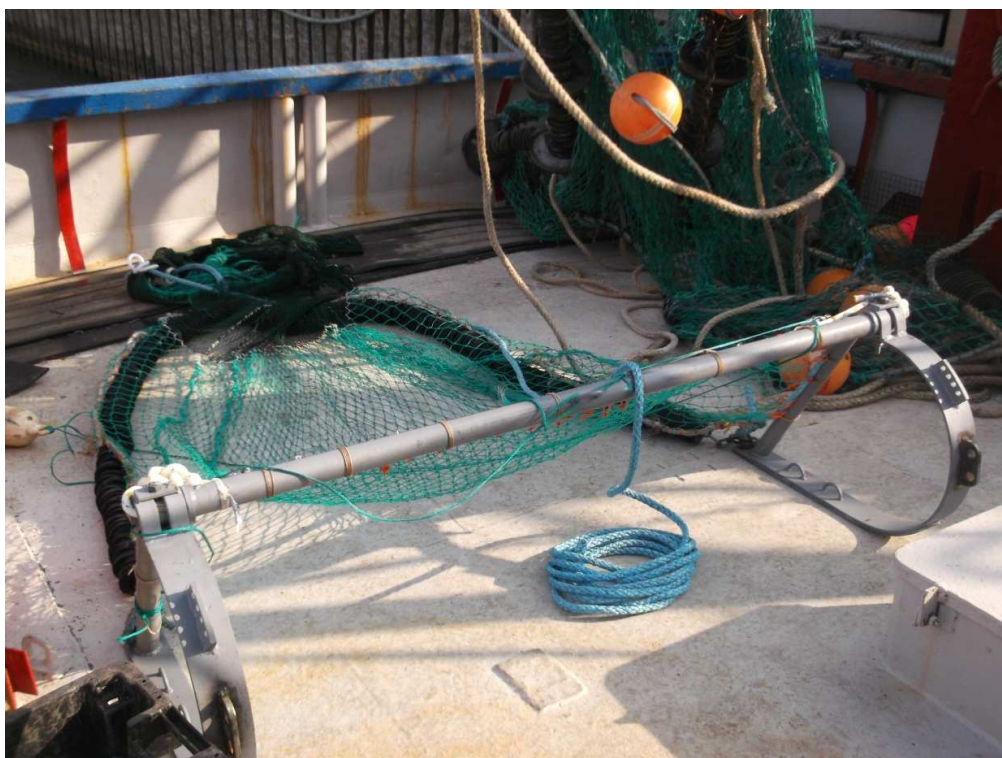
Plate 3. Standard design beam trawl used in the surveys
