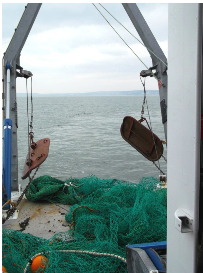
Plate 2. Otter trawl ready to be lowered into the water
