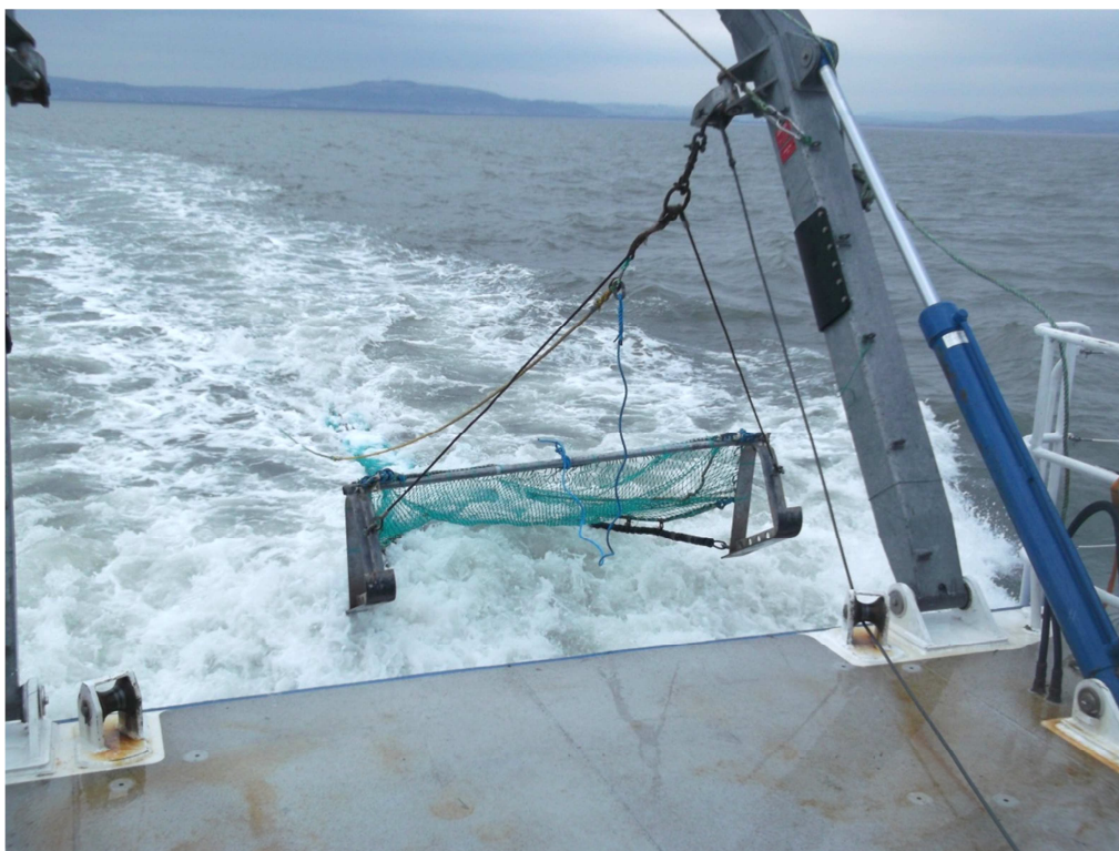
Plate 3. Standard design beam trawl ready to be lowered into the water
