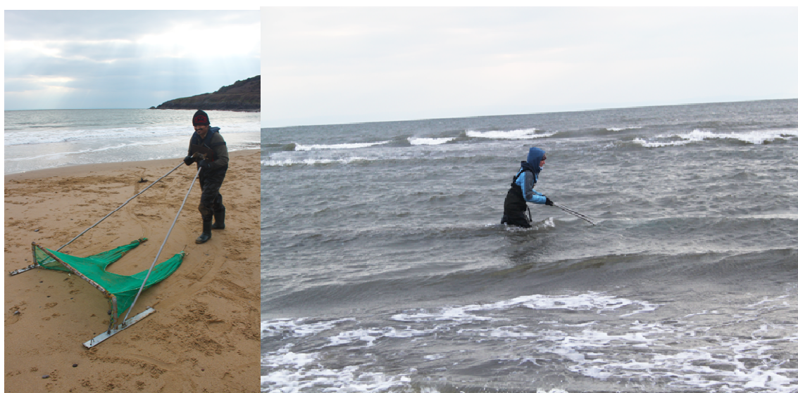
Plate 1. Riley net design and technique utilised during sampling
