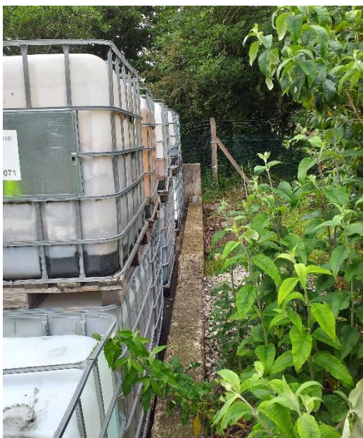
Lack of separation between stored IBCs and adjacent gravel surfacing
