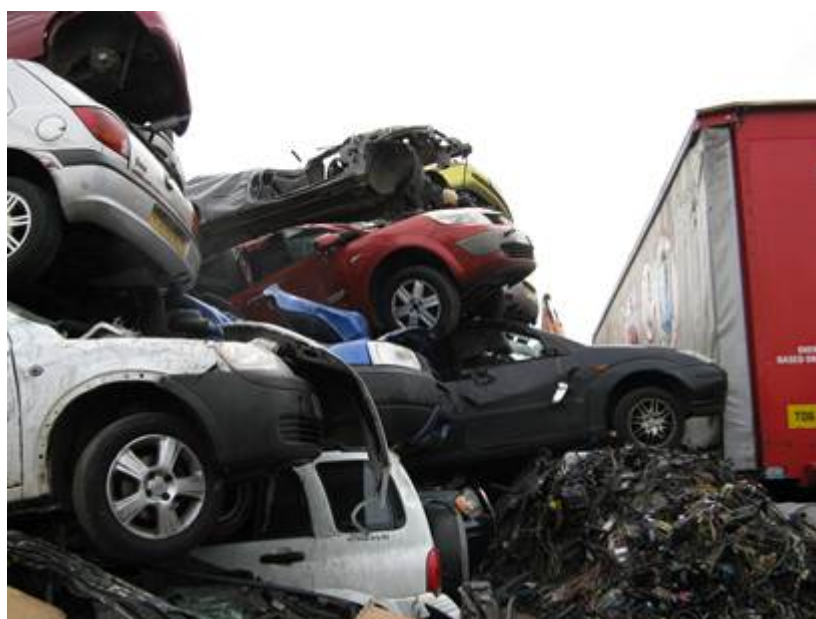
Photo showing part depolluted ELVs awaiting crushing/baling.
