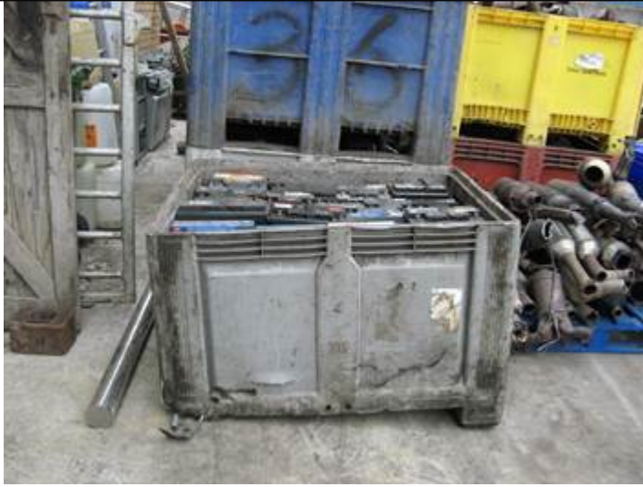
Photo showing battery box containing batteries while uncovered and with large cracks on the side of the box.
