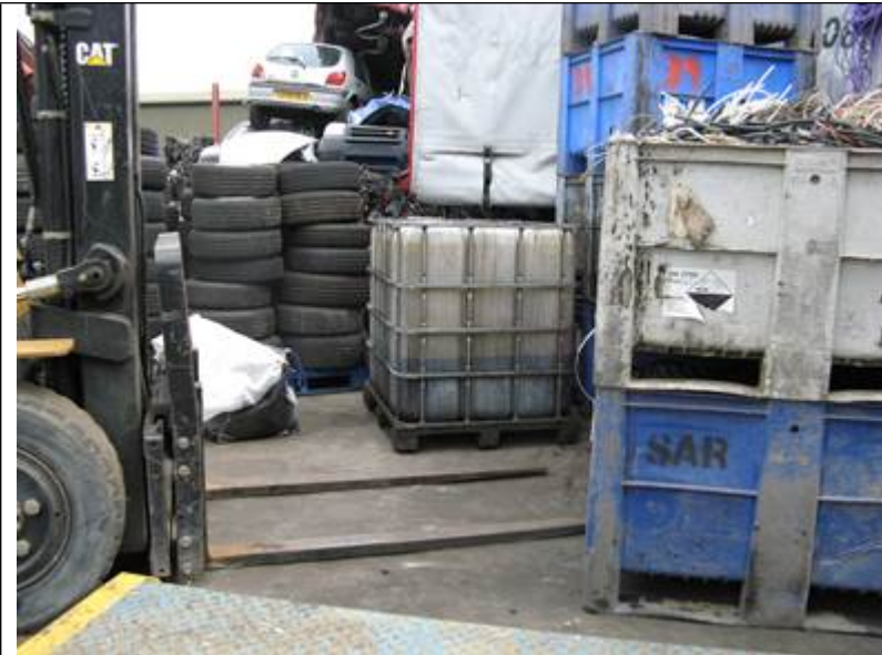
Photo showing IBC where separately collected fluids (engine, gear box oil etc) are mixed and stored without any secondary containment.
