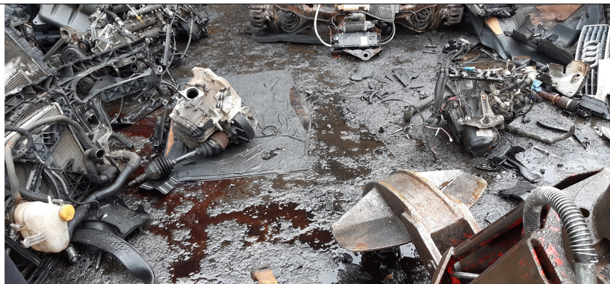
Photo 1 - Pooling of oil on flooring with no countermeasures in place
