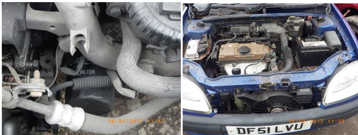
Oil filter and battery observed in (separate) vehicles
