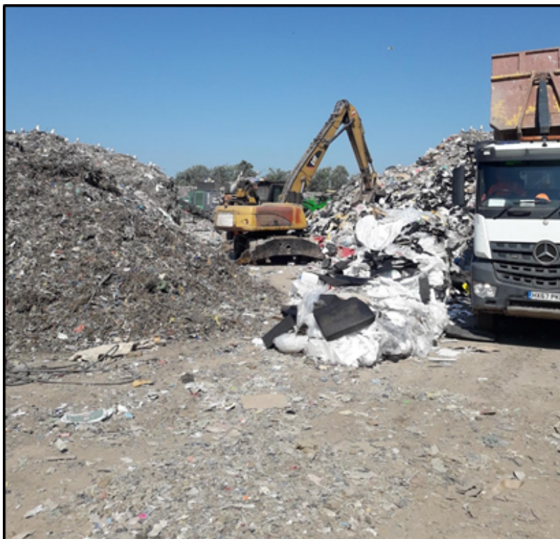
Photograph 5 | taken on 15/07/19 - showing mixed waste deposited on Field 1 within the fire breaks between RDF stockpiles
