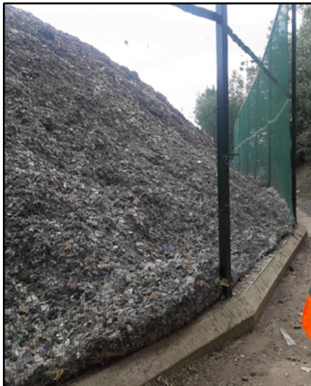
Photograph 4 | taken on 10/07/19 - showing material stored in the Transfer Station pushed against the mesh fencing
