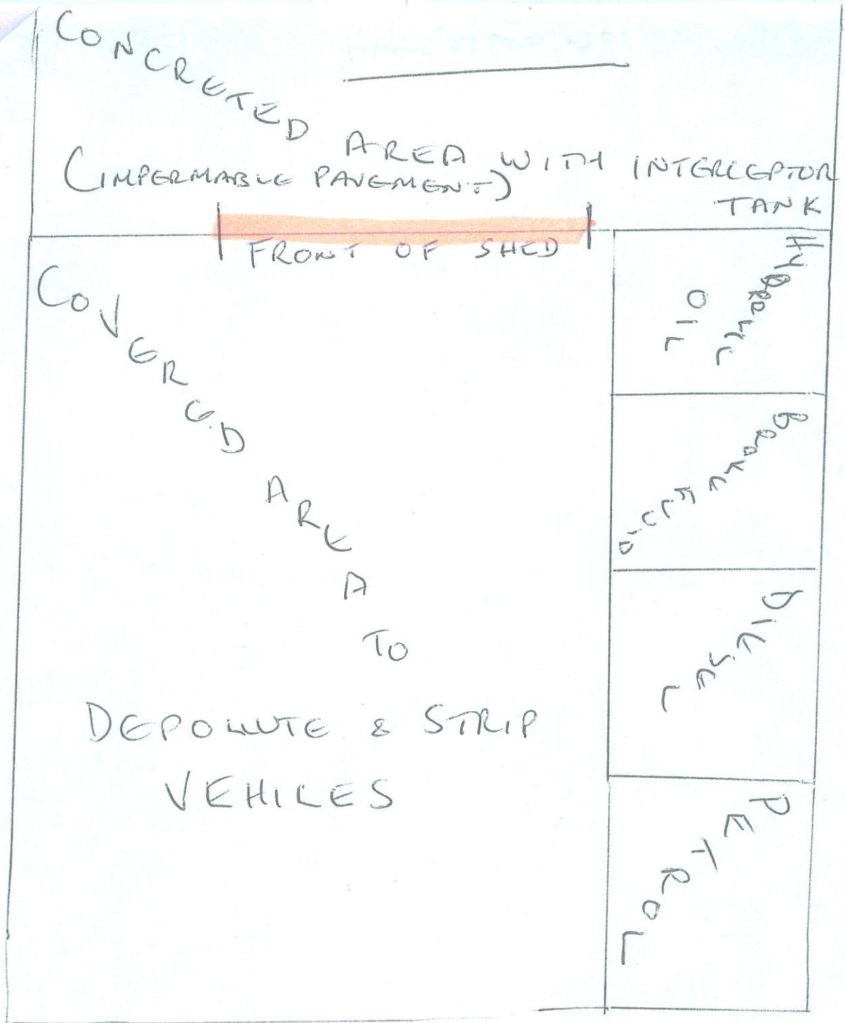
\* THIS IS THE PLAN FOR OUR STRIPPING SHED.
