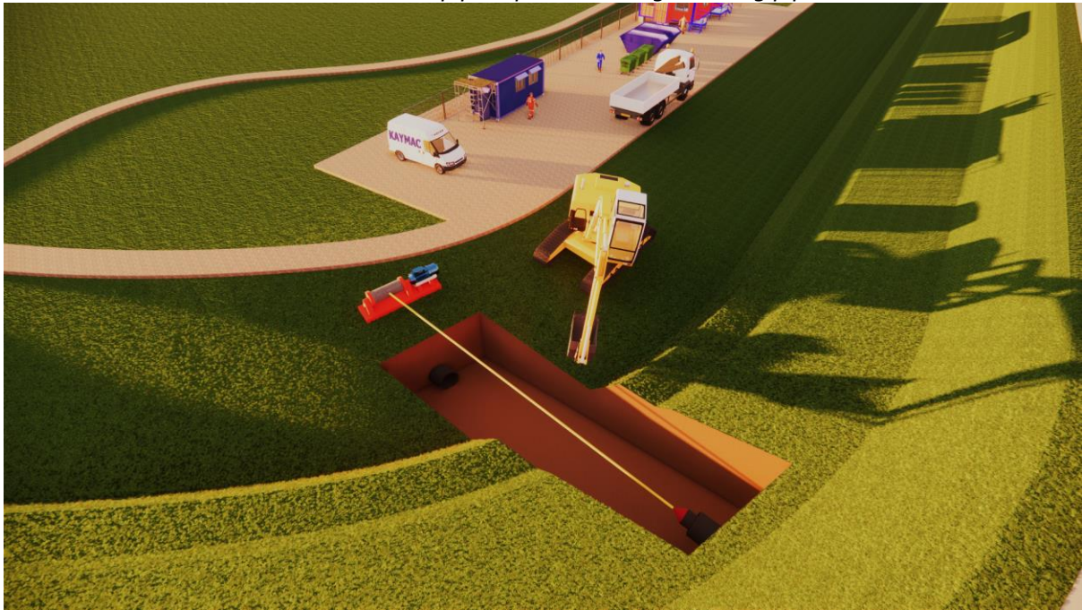
New 355mm OD pipe slip-lined through to the landward side of the sea defence wall.
