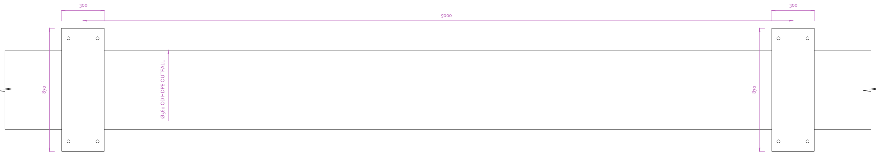
CONCRETE BALLAST COLLAR DETAILS
