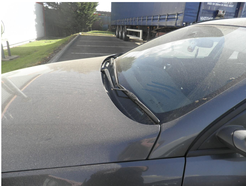
Dust deposited on neighbouring vehicles
