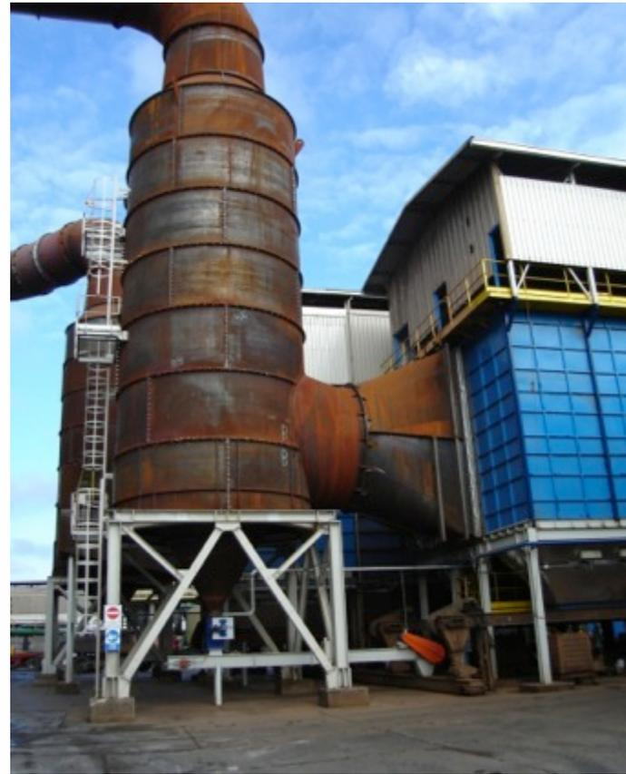
Revamping of dedugsting plant for EAF line and insertion of vertical preseparator cyclones
