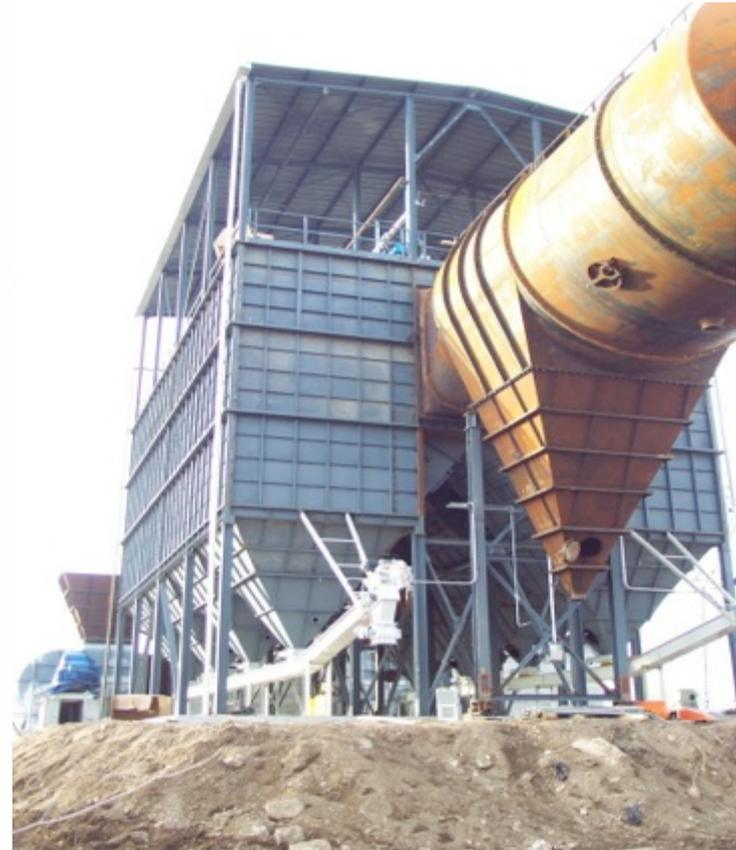
Pulse jet bag filter, evaporating cooling chamber, exhaust fans, axial cyclone
