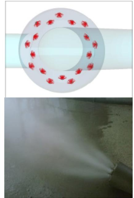
The second type is with dual fluid, water and compressed air: with this type of nozzles the water drops are smaller, though the evaporation time is shorter. The result is a smaller GCT, but with higher operating costs.
