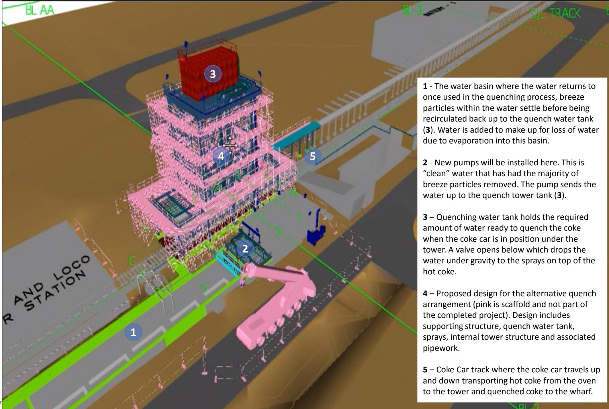
**1** - The water basin where the water returns to once used in the quenching process, breeze particles within the water settle before being recirculated back up to the quench water tank (**3**). Water is added to make up for loss of water due to evaporation into this basin.
