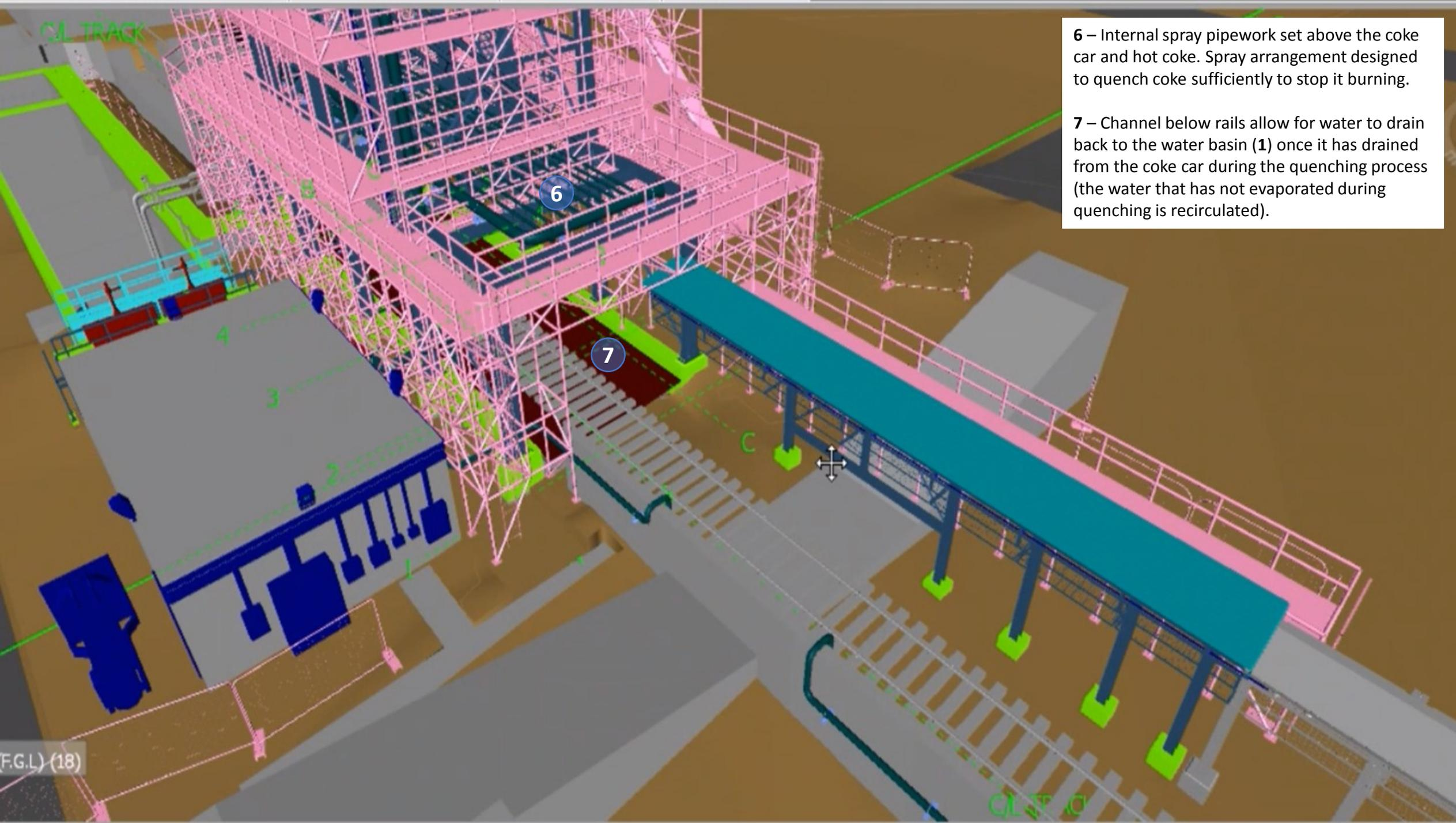
**6** – Internal spray pipework set above the coke car and hot coke. Spray arrangement designed to quench coke sufficiently to stop it burning.
