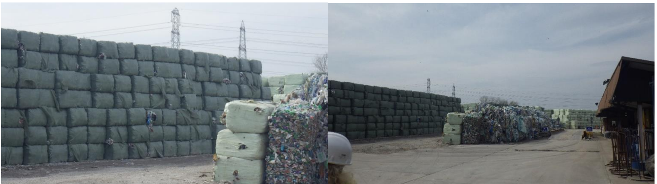
Baled RDF on site ( Some stored on Impermeable ground), some of the wrap on the bales is damaged.
