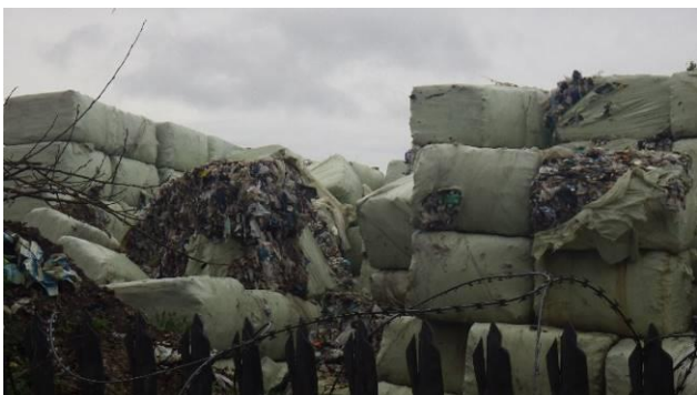
Photograph 3. Damaged baled RDF
