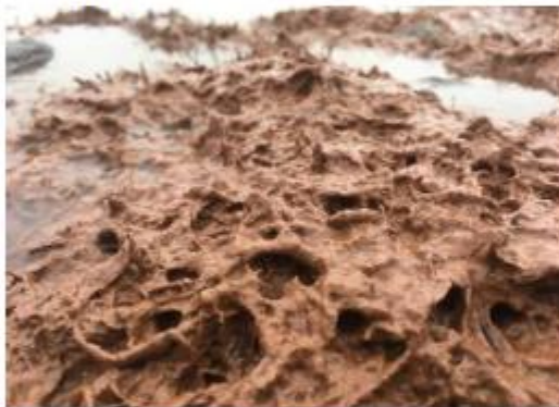
Close up FlocMat showing accretion of silt
