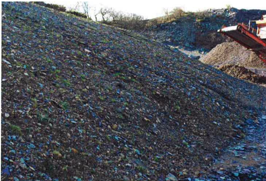
Plate 2: Previously-restored land at Ty Mawr West using waste arising from slate waste reprocessing operations which generally contains soil-forming materials. No seeding has been undertaken on this area which is beginning to revegetate naturally.
