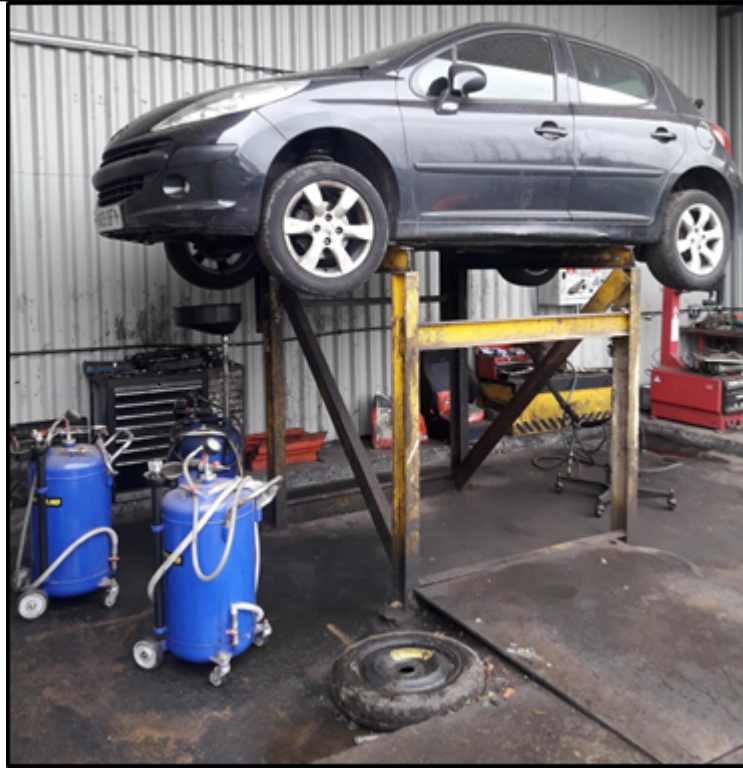
Picture 1 – showing vehicle depollution bay. Punctured oil tank draining into container – taken 11/06/19
