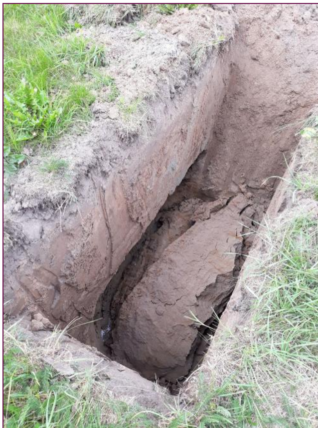
Photograph 5: TP224, example of general sand unit underlying the site with base collapsing.
