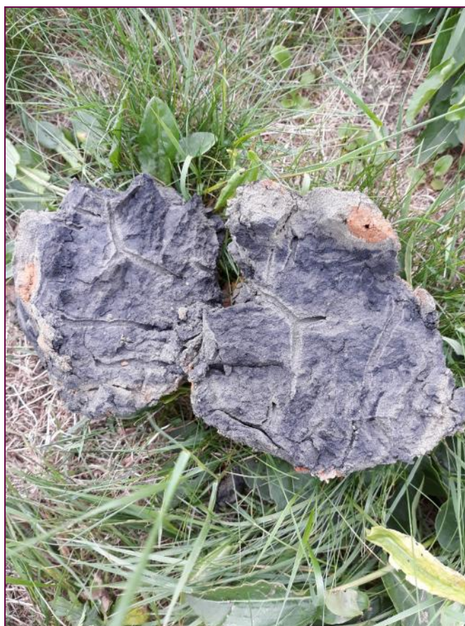
Photograph 6: TP223, example of sandy clay horizon.
