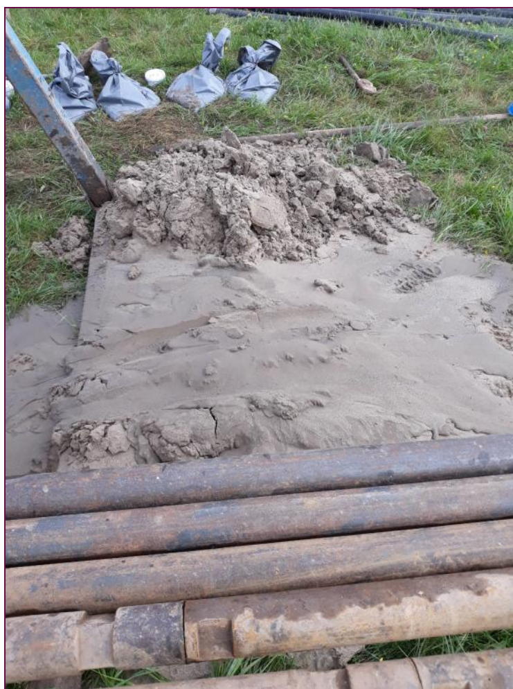
Photograph 2: CP206, general view of sand drilling returns.
