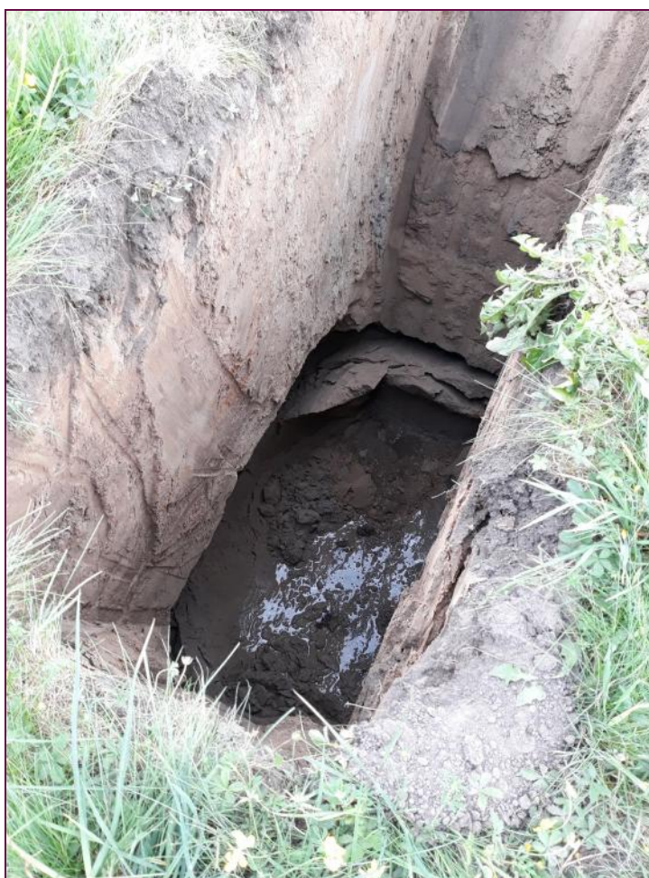
Photograph 8: TP225, water ingress at the base of the pit.
