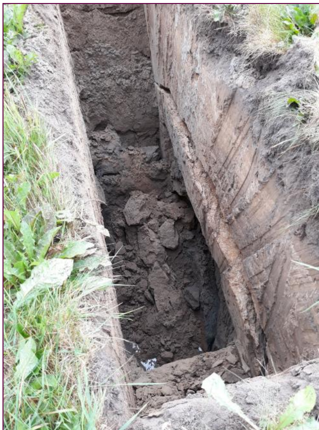
Photograph 3: TP232, example of general sand unit underlying the site.
