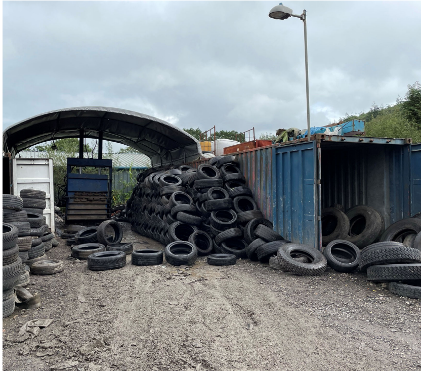
Plate 2-2 Unloading and interlacing of tyres adjacent to baler
