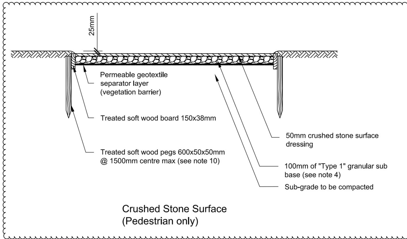
Crushed stone surface detail to be used for Honddu Forge
