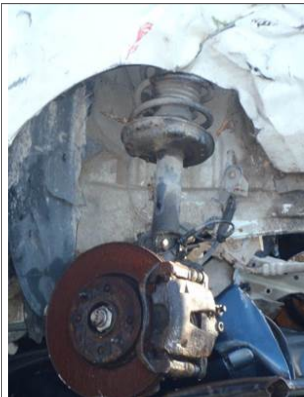
Image 2 – Example of non-de-polluted vehicle found on site, with shock absorbers still intact.
