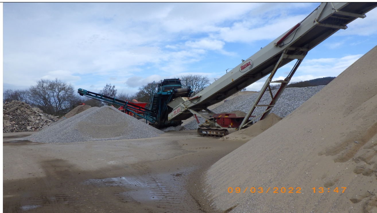
Photograph showing screener and conveyor separating sand and pebbles into stockpiles
