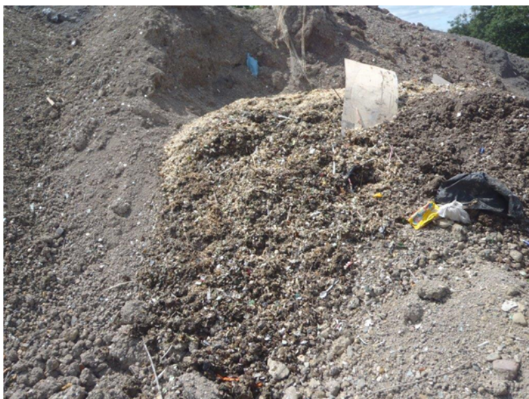
Trommel fines – oil contaminated waste
