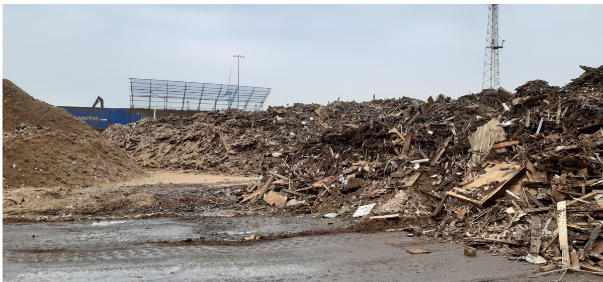
Photo 2 - Wood stockpiles within 4 metre recommended maximum height
