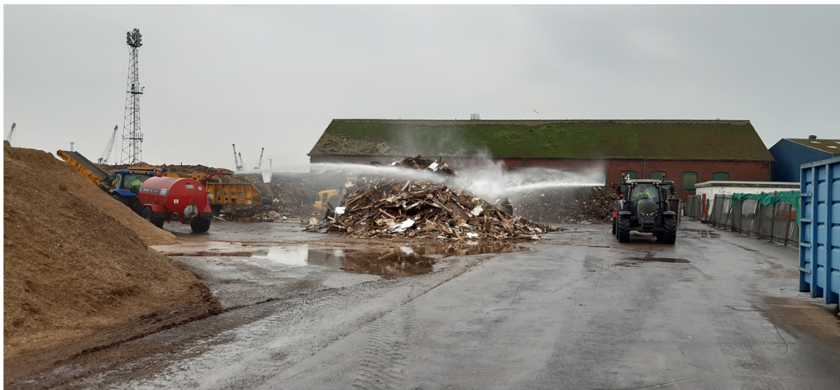
Photo 3 - Demonstration of water cannons on unignited wood stockpile
