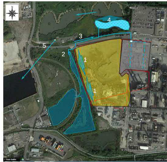
Figure 1.2 – Conceptual Landfill Capping Design – Drainage (Amended from Slide 17: Landfill Closure Summary Presentation, 1st March 2018)
