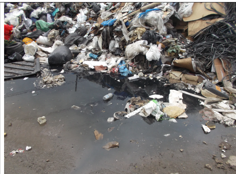
Picture 1 - showing discoloured leachate pooling around mixed waste in stored in work Area A
