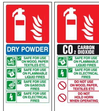
Figure 2: Fire Extinguishers Type and Application
