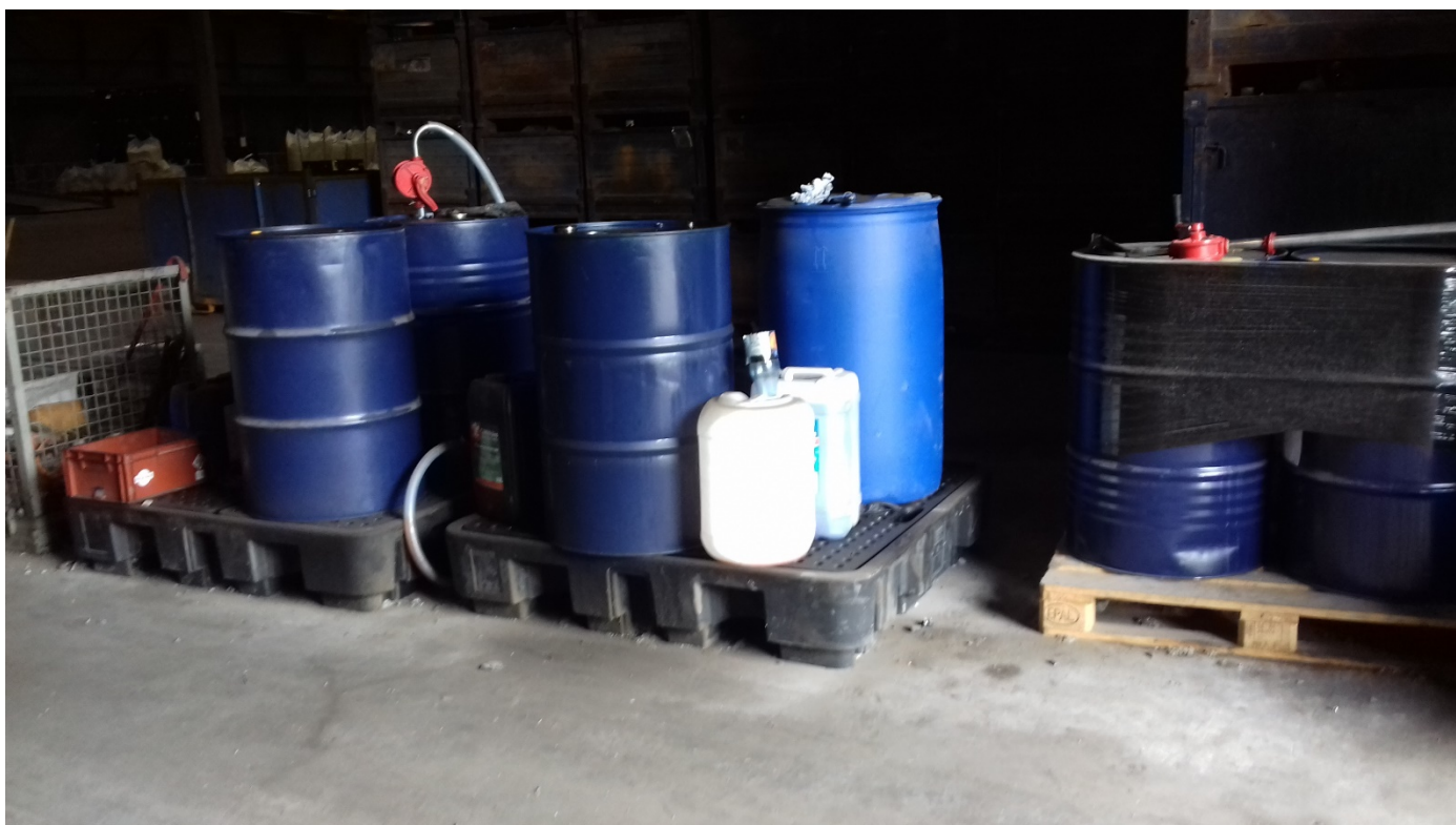
Plate 5: Temporary storage on mobile bunds of chemicals / maintenance oils, lubricants etc.
